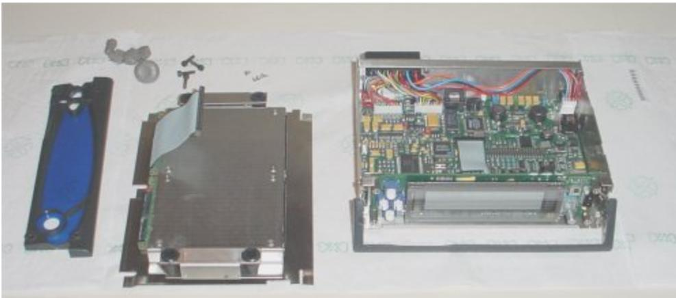
Next, remove the drive tray assembly (two screws on either side of the player).
