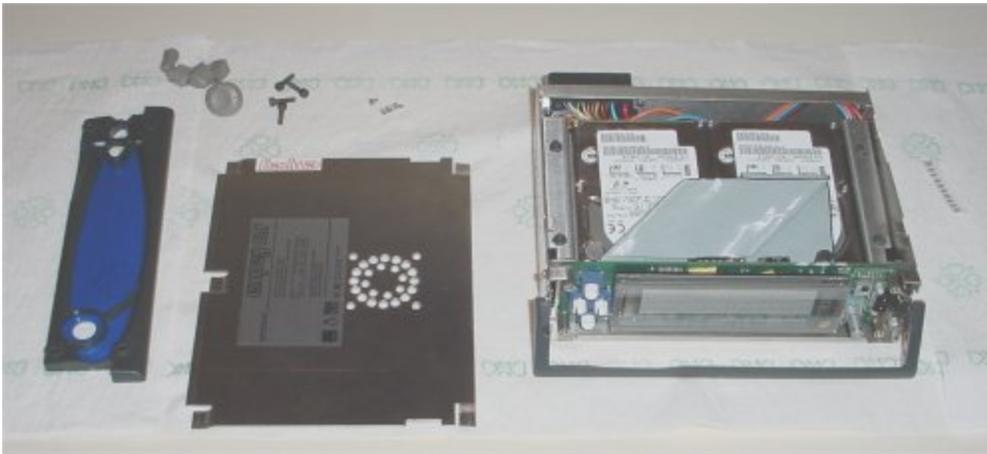
You will need to remove the face (four Allen head screws), pop the knobs and buttons off, slide off the lens, and then remove the player cover.
