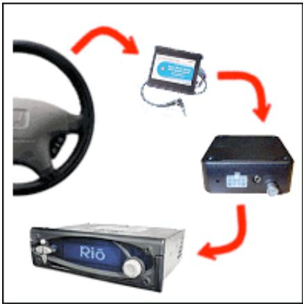
These are third-party integration devices designed to connect factory steering wheel controls directly into the "stalk port" on Sony-brand stereos. If one exists for your model of car, then these will also plug into the add-on tuner module for the Rio Car. [Soundgate](#) is one company that makes this type of interface for Ford and GM vehicles.
