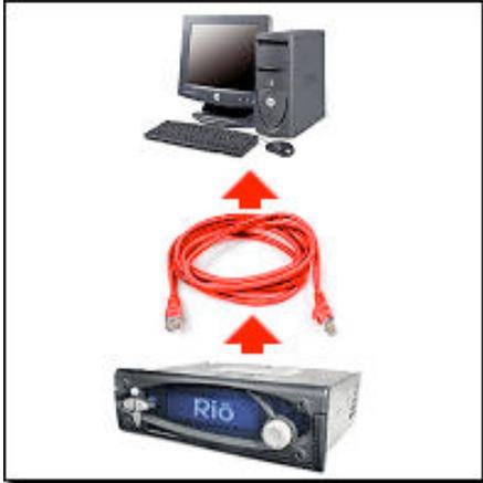
If you don't have a hub, and you don't have any reason to connect your computer to other computers or to a broadband internet link, you can use this method to connect the car player directly to your PC's ethernet card. I don't recommend doing this, since hubs are dirt-cheap and can be found at any computer store. Hubs allow you to connect multiple computers to the same network and take advantage of [all of the features networks have to offer](#).
